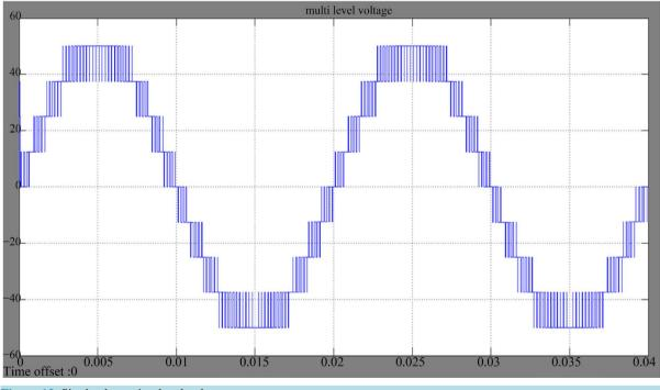
Figure 12. Single phase nine-level voltage output.
