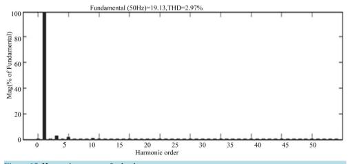
Figure 15. Harmonic spectrum for load current.
