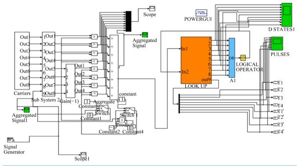
Figure 9. Proposed D-state switching scheme.
