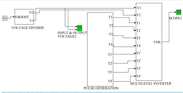
Figure 11. Overall simulation model for nine- level inverter.
