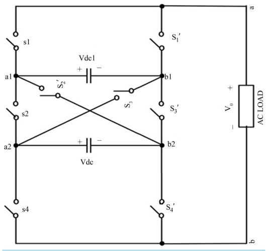
Figure 2. Proposed single phase nine-level inverter.
