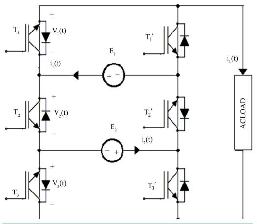
Figure 1. Single phase nine-level inverter based on switched dc source topology.
