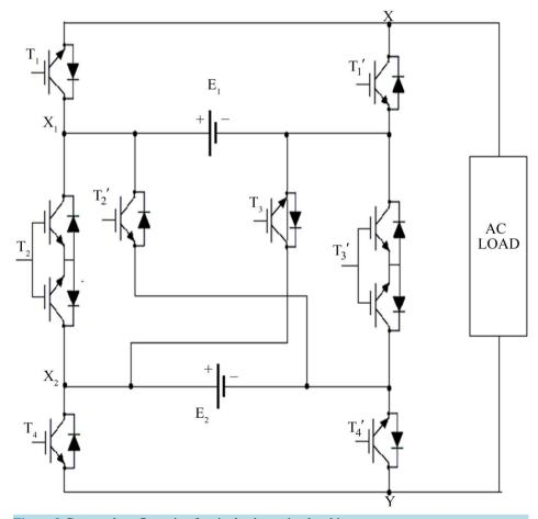
Figure 3. Proposed configuration for single phase nine-level inverter.
