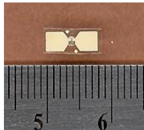
Figure 3.13b: RFID IC in strap form, with reference scale.
