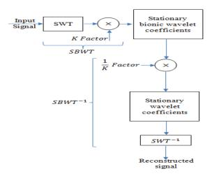
Figure 1. The applications of (SBWT) and its inverse, SBWT<sup>-1</sup>.
