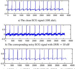
c) The denoised ECG signal (SNRf = 18.714938dB, PSNR = 36.418703 dB, CC = 0.993442, MAE = 0.011001, MSE = 0.000228
