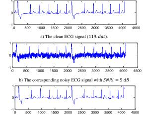
c) The denoised ECG signal (SNRf = 14.758179dB, PSNR = 29.715380dB, CC = 0.983566, MAE = 0.019725, MSE = 0.001068).
