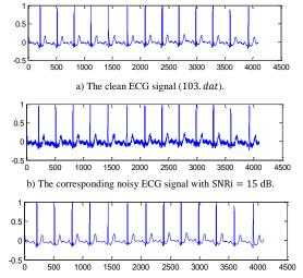
c) The denoised ECG signal (SNRf = 22.581725dB, PSNR = 39.240232 dB , CC = 0.997524, MAE = 0.007968, MSE = 0.000228).
