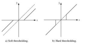
Figure 3. Illustration of two Types of thresholding function.
