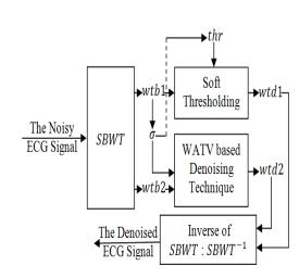
Figure 2. The flowchart of the proposed ECG denoising approach.
