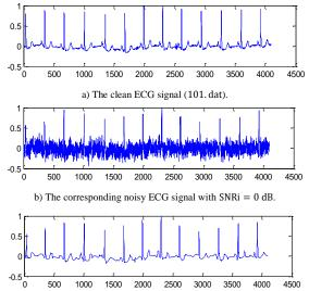
c) The denoised ECG signal (SNRf = 12.276751dB, PSNR = 30.590276dB, CC = 0.970692, MAE = 0.021001, MSE = 0.000873).
