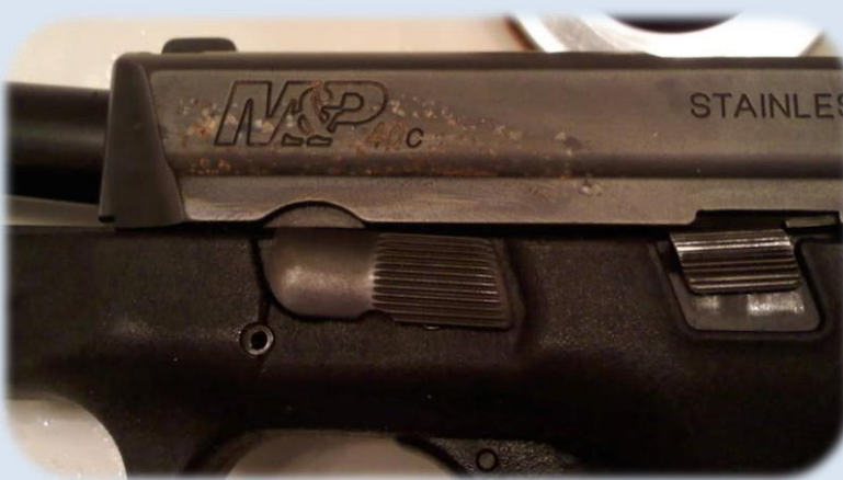
A Smith & Wesson M&P40C pistol showing surface rust. )
