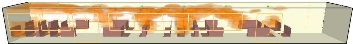
Figure 6b: FDS predicted fire suppression, 540s from ignition (scenario 2)
