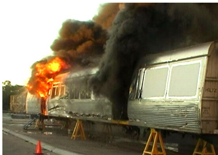
Figure 5: CSIRO train fire experiment
