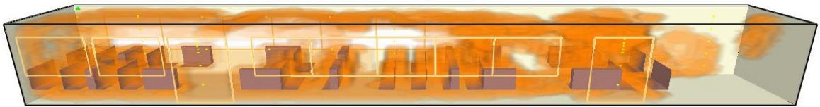
Figure 6a: FDS predicted fire growth– no suppression, 560s from ignition (scenario 1)
