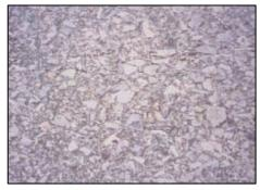
smooth. It is caused by naturally smooth, non-crushed gravels and/or crushed rock that wears down quickly under action of traffic. It requires covering the surface with a asphalt pavement treatment that has good frictional characteristics. *Photo courtesy of US DOT*.
