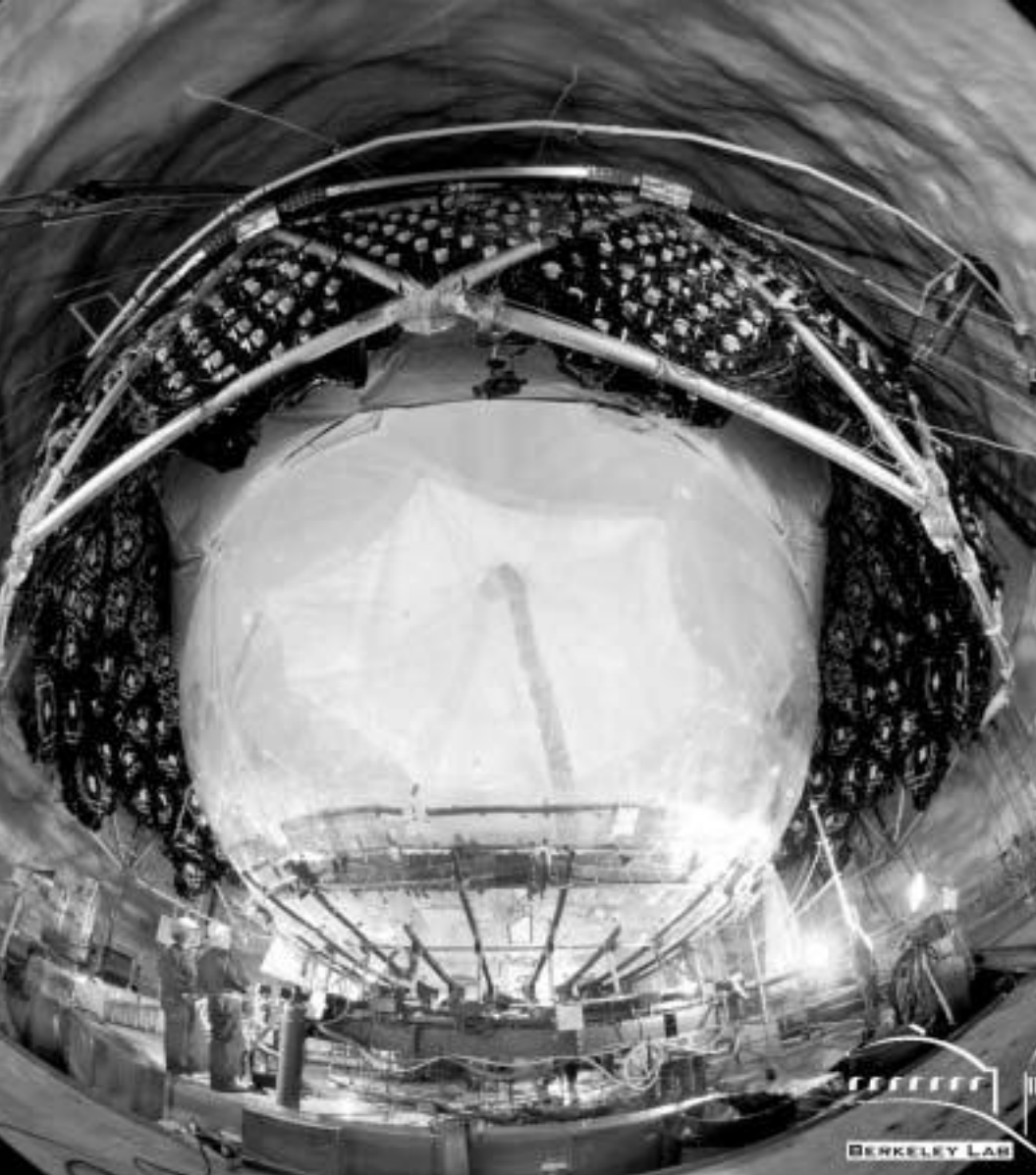
The SNO detector just before completion of the bottom of the acrylic vessel. The acrylic used for this vessel is over 2.5 inches thick and built to hold 1000 tons of heavy water.
