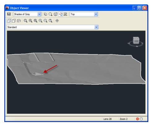
6. When you are finished viewing the surface close the object viewer window to return to the drawing editor. You should also be able to identify this hole by looking at the contours in plan view.
