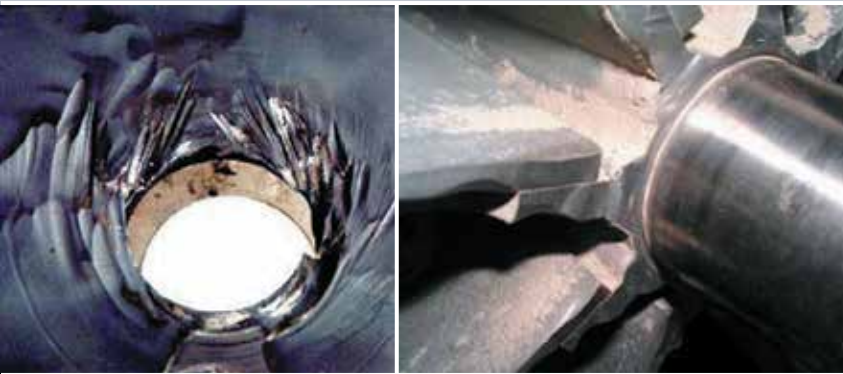
Images show wear through High Velocity Erosion
