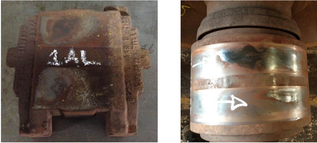
Figure 39: Indications of Uneven Loading in the Wear Patterns on the Adapter Crown and the Outer Diameter of a Cup
