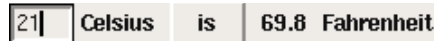
Fig. 4.1 Screen dump of the graphical interface for a Celsius to Fahrenheit conversion program. The user can type in the temperature in Celsius degrees, and when clicking on the is button, the corresponding Fahrenheit value is displayed.
