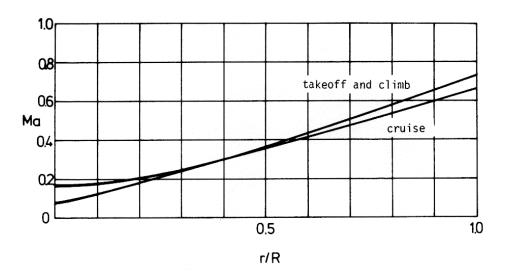
Figure 4: Mach numbers on the propeller blade for cruise and takeoff conditions.
