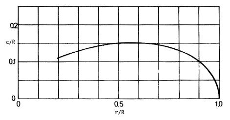
Figure 3: Resulting chord distribution of the designed propeller.
