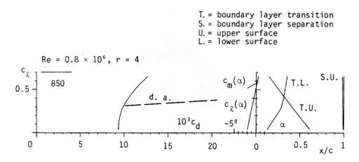
Figure 6: Drag polar of Profile 850 for M = 0.74.
