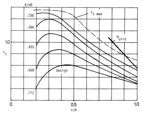
Figure 2: Lift coefficients c<sub>1</sub> on the propeller blade for various pitch angles and advance ratios.
