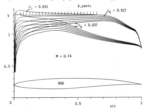
Figure 5: Profile 850 for the propeller tip r/R = 1 with velocity distributions for M = 0.74.
