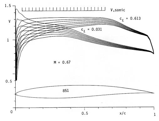
Figure 7: Profile 851 for r/R = 0.9 with velocity distributions for M = 0.67.
