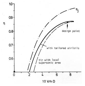
Figure 11: Propeller efficiency against advance ratio.
