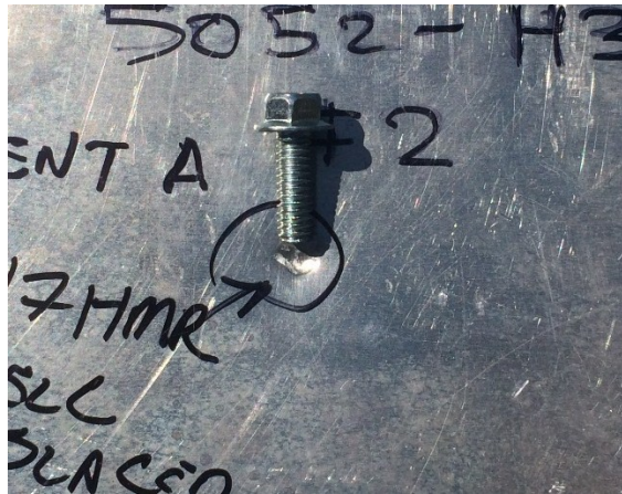
Figure 41 Largest dent obtained from ballistic pendulum testing
