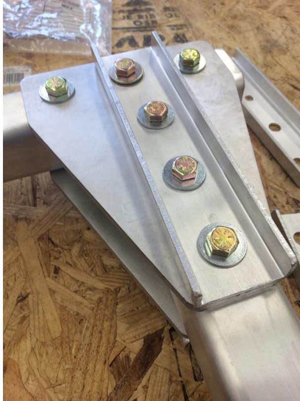
Figure 31 Gusset for rear vertical member of the test stand illustrates most of the details of the frame's construction
