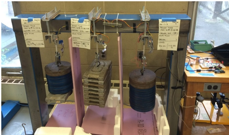
Figure 24 Stress Rupture Test Rig
