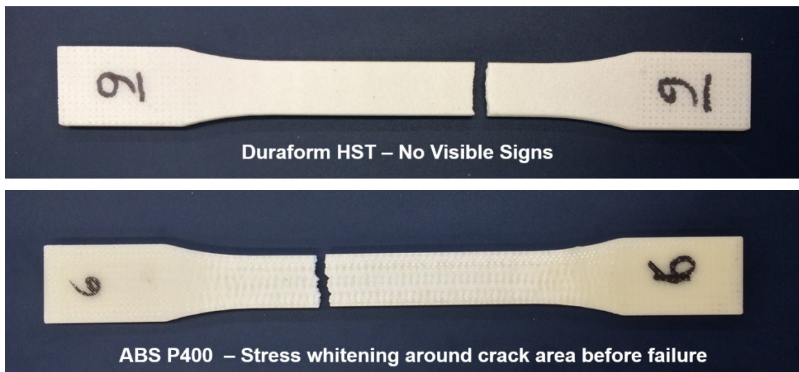
Figure 23 Comparison of failed P400 and Duraform HST dog bones
