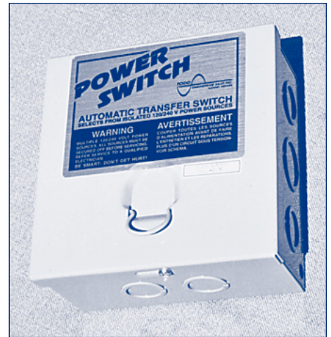
The Todd TS-30 has a 20- to 30-second time delay to let the generator warm up.
