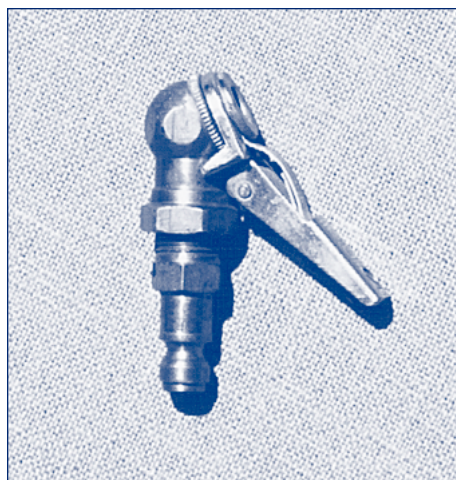
A clip-on chuck can be used to access an Electro Level II system.
