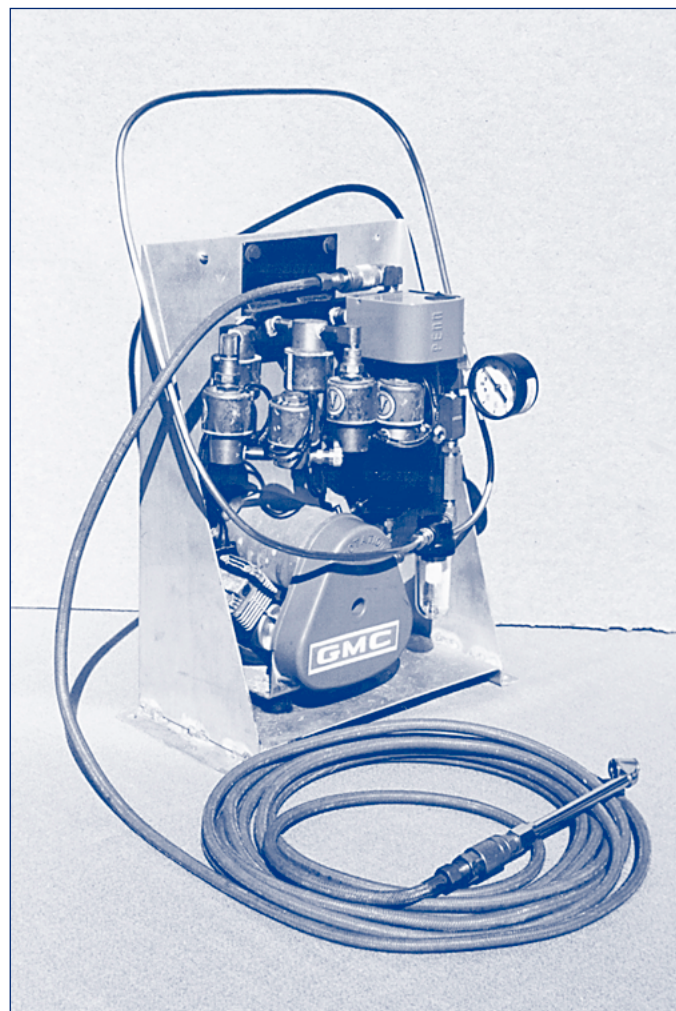
An upgraded Electro Level I module with a quick coupler, copper air-cooling loop, stainless-steel check valve, 5-micron filter, pressure-relief valve, pressure gauge and brass air-brake fittings. A dual-foot inflator is attached to a 25-foot air hose.
