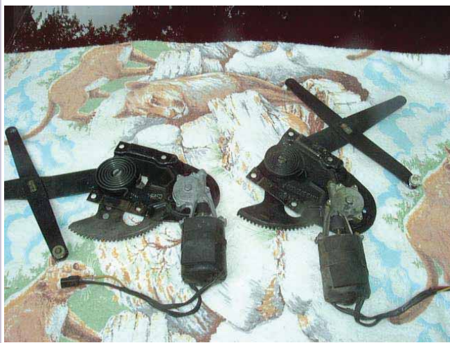
Window Motors and Gear Train ready to be installed after a Thorough Renovation.
