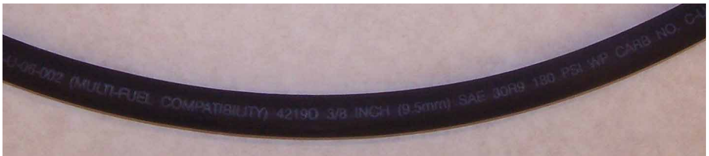
Standard Fuel Injection Hose illustrating typical markings. Note the PSI rating and SAE30R9 indications.
