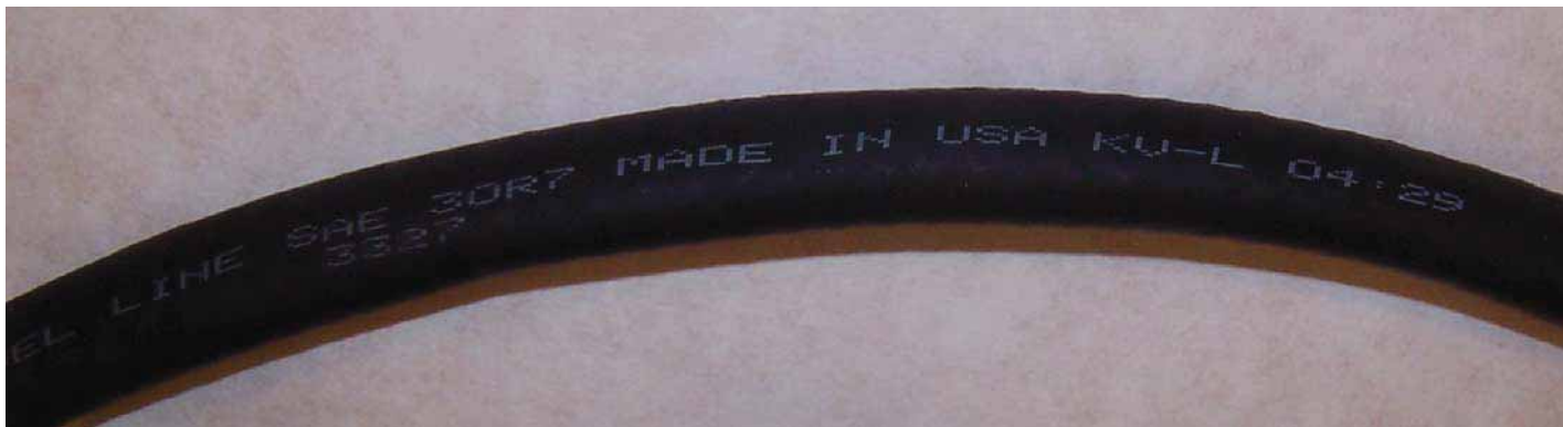
Regular fuel line, SAE30R7, that IS NOT Ethanol resistant. Found in classics routinely as that was the right hose for that era.
