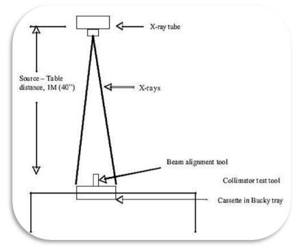
Figure 6. Collimation/ Beam alignment setup.
