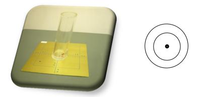
Figure 4. Beam Alignment Test Tool.
