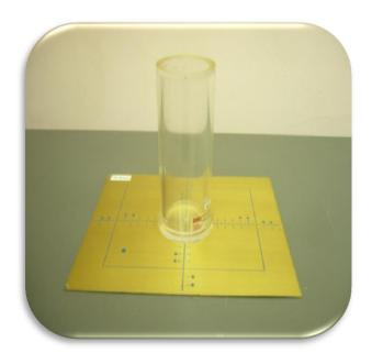
Figure 12. Collimator/ Beam Alignment test tools.
