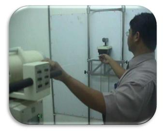
Figure 9. Leak test at 1-meter distance.
