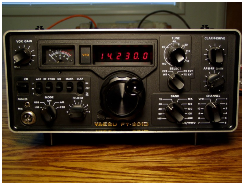
Figure 7: FT-301D with the new PB-1542B-R display installed
