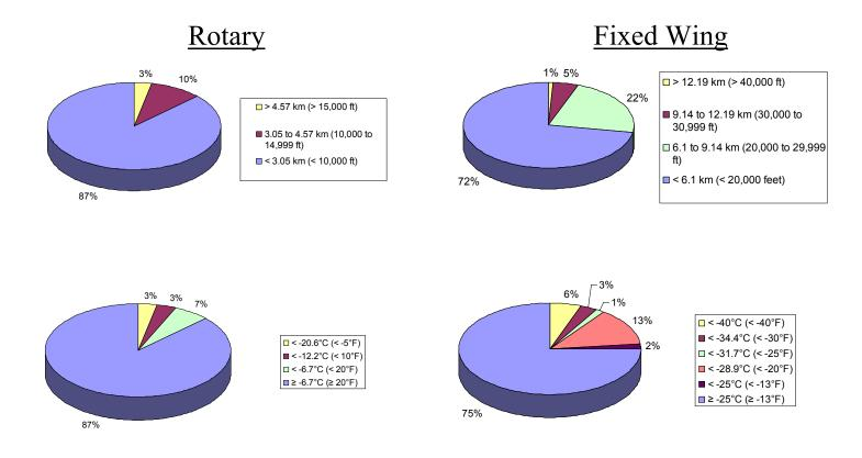
Figure 22. Summary of OAT and Altitude Conditions at Nacelle Fire Suppressant Release
