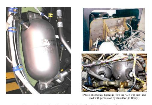
Figure 7. Engine Nacelle/APU Fire Bottle Installations
