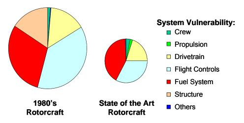
Figure 31. Notional Reduction in Aircraft Vulnerable Area
