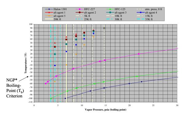
Figure 11. Suppressant Boiling Point vs. Standard Atmosphere Pressure
