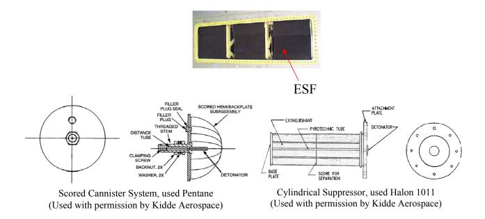
Figure 34. Examples of Fuel Tank Ullage Fire/Explosion Protection Techniques
