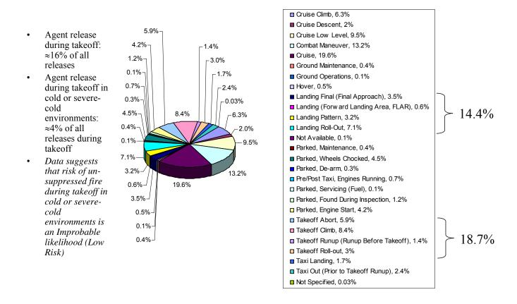
Figure 25. Fixed-Wing Fire Incidents and Mishaps
