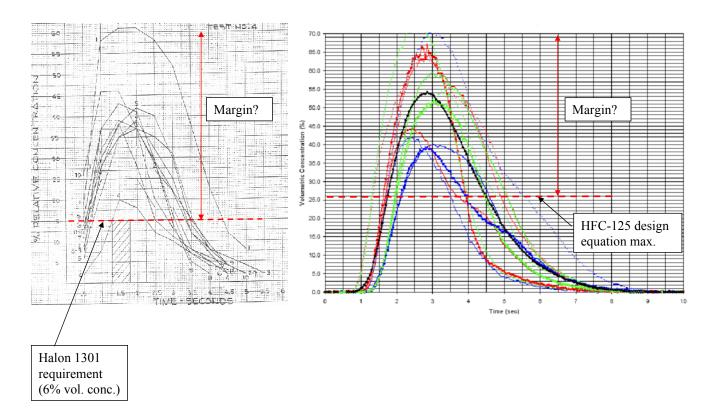
Figure 27. Example Nacelle Fire Suppression Systems Certification Concentrations
