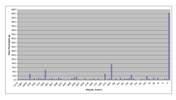
Figure 21. In-Flight Suppressant Deployment vs. Altitude, DoD Data, 1980-2002
