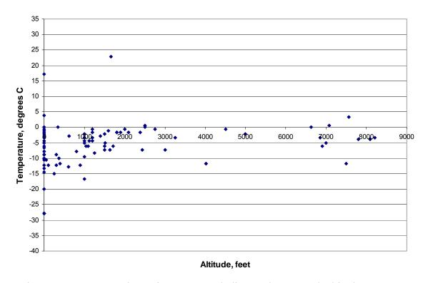
Figure 12. NTSB Database Fire Events Including Both OAT and Altitude, 1988 - 2000
