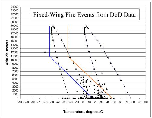
Figure 18 DoD Aircraft Fire Events vs. Flammability Profiles
