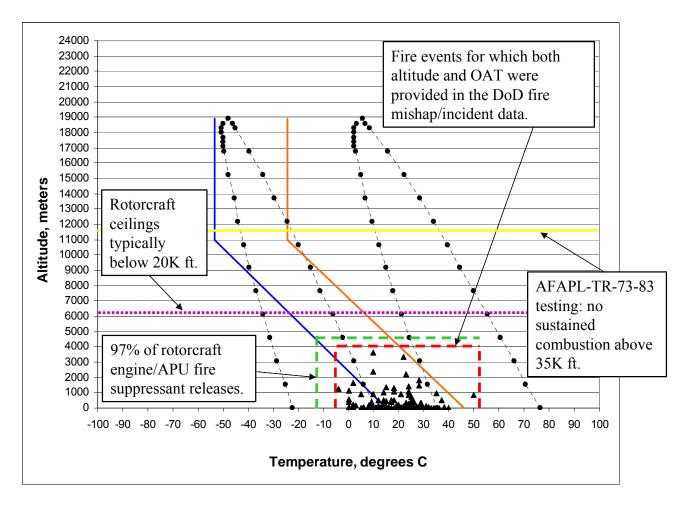
Figure 23. DoD Rotary Aircraft Fire Data versus Atmospheric Profiles, Flammability Limit Profiles, Operational Ceiling, and Suppressant Release
