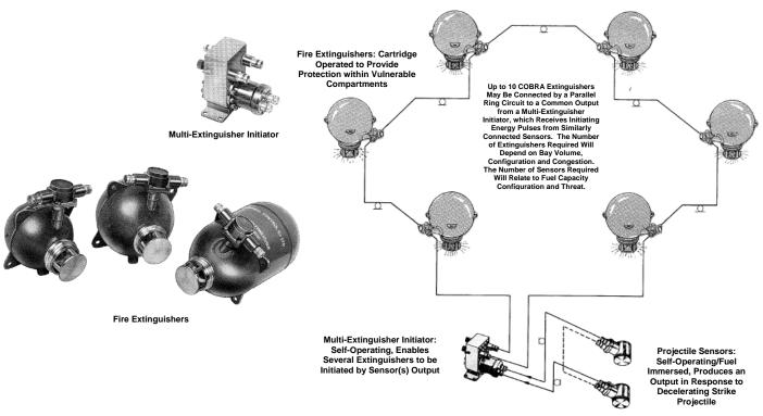
COBRA system - components interconnection diagram
