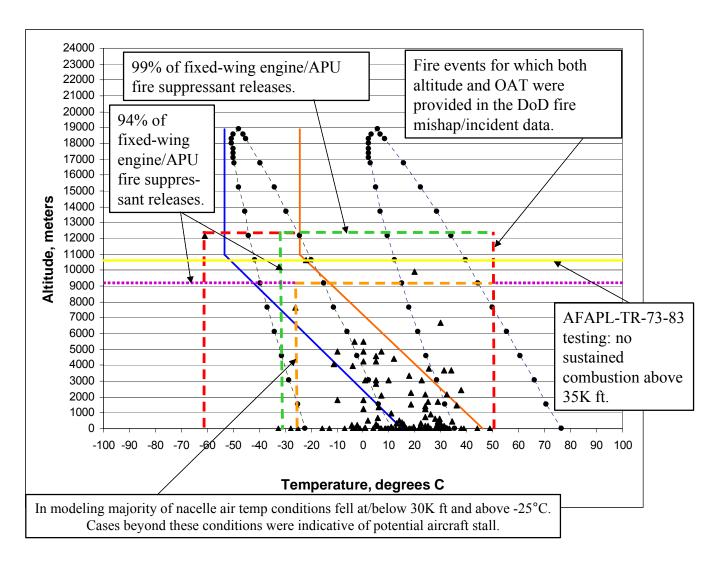
Figure 24. DoD Fixed-Wing Aircraft Fire Data versus Atmospheric Profiles, Flammability Limit Profiles, Potential Stall Condition and Suppressant Release
