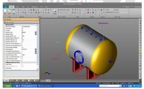
Fig.2. Vessel Geometry in PV Elite.
