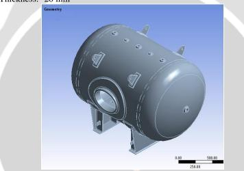
Fig. 3. Model of Air Receiver.
