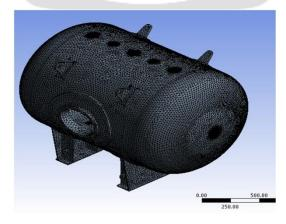
Fig.-4 Meshing of Equipment
