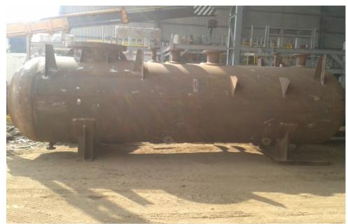
Fig.1. The typical horizontal storage vessel design
