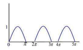
The function f(t) is of period  $T = 2\pi$ . The Laplace transform of f(t) is
