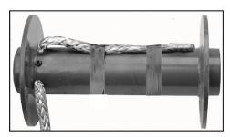
For Synthetic Rope a common method of installing a synthetic rope is through a hole in the drum coming from underneath the drum using enough line so it reaches opposite end of drum. Position the
