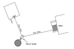
**Figure 9.** illustrates the use of a pulley block to change the direction of the pull. The pulley block is attached to an anchor point with a nylon strap and shackle, and the winch rope is redirected to the load.
