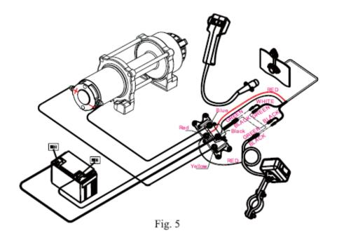
4. Check the rotating direction of the drum. Pull and turn the clutch knob to the "off" position (drum can be turning free). Pull out some cable from the drum, and then turn the clutch knob to the "in" position. Press the "cable out" button on the handheld switch, if the cable is releasing then it is connected the right way.
