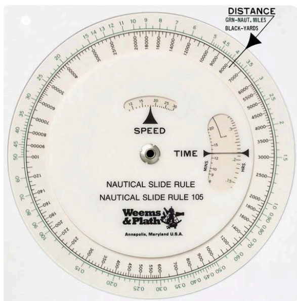
Figure 3.9. Nautical slide rule.
