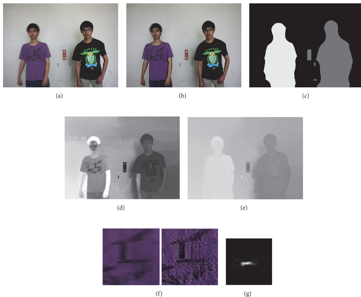
FIGURE 14: Deblurred result of image “Students.” (a) Blurred image with nonuniform motion blur. (b) Deblurred result. (c) Clustering result. (d) Zhuo’s defocus map. (e) Proposed uniform defocus map. (f) Close-ups of (a) and (b). (g) PSF corresponding to moving student as shown in (a).
