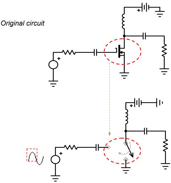
Ideal-switch model of transistor:
