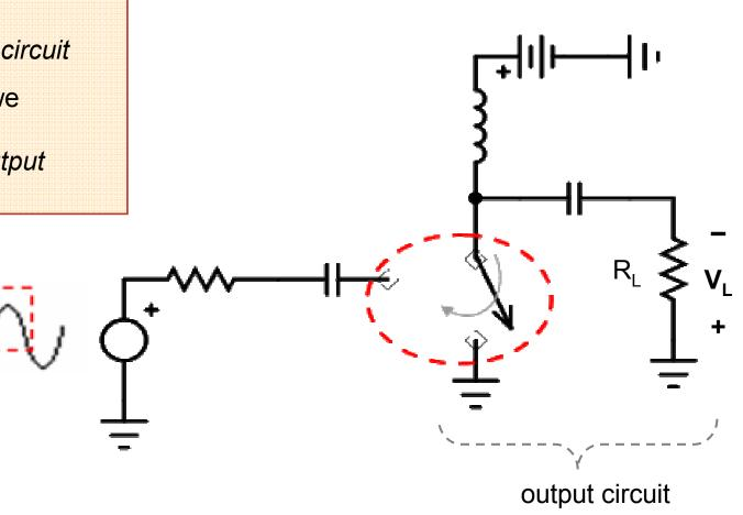
Analysis of Idealized Class C Amplifier – Output Voltage Waveform
