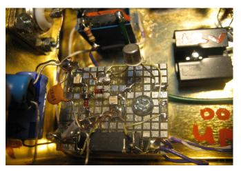
RF Sensor for T/R Switching
