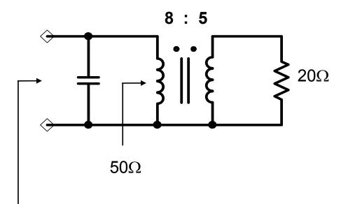
for evaluation of match, connect antenna analyzer here
