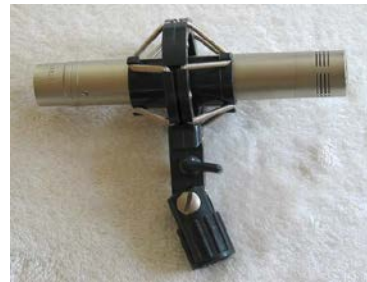
Schoeps CMC5 with MK41 capsule with mount to attach to a boom
