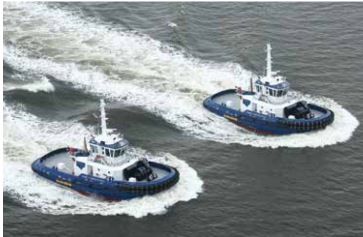
Signet 82-Metric Ton Bollard Pull Z-Drive tug boats
