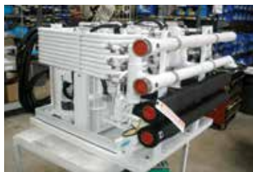
Marine Air two-stage chiller under construction at the Dometic Marine manufacturing facility
