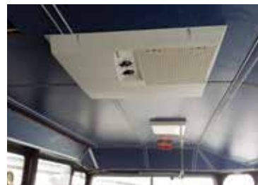
The DuraSea Air Distribution Box with controls and return air in the pilot-house of the Bahamas Ferries Sealink catamaran.
