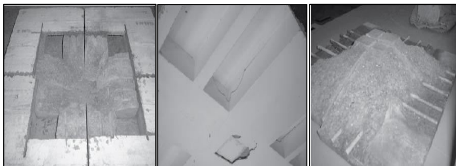
a. Loss of failure b- Punching failure surface c- Punched out piece
