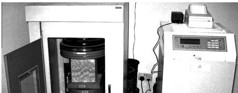
Figure 1 Compression test set-up.
