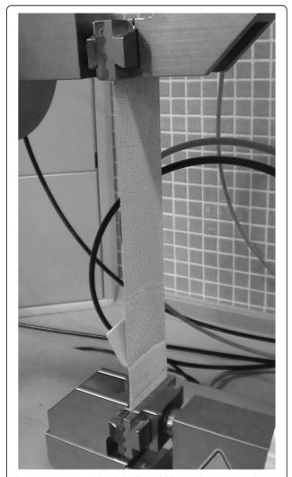
**Fig. 2** Dynamometer Zwick/Roell. model Z005 (Ulm. Germany) during the adherence test of one red tape. The tape is adhered on a piece of untanned sheepskin
