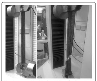
**Fig. 1** Dynamometer Zwick/Roell. model Z005 (Ulm. Germany) during the strain test of one black tape. The appearance of white marks in the tape indicates its immediate breakage
