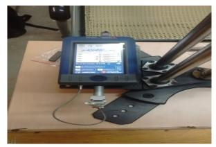
Figure3 Surface Roughness tester
