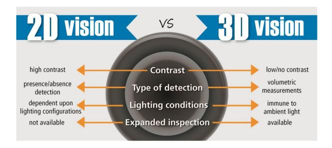
Compared to traditional 2D vision systems, high-speed 3D vision systems provide value to tire manufacturers in the following ways:
