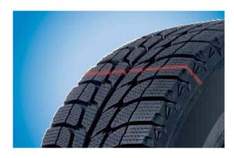
principle requires the presence of a known angle between the laser and the camera's receiving element. For a specific angle, the position of where the sensed laser light appears on the receiving element determines the measured height of the target object.
