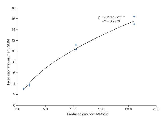
Figure 3 Fixed capital investment as a function of the produced gas flow. MM, million; MMscfd, million standard cubic feet per day.
