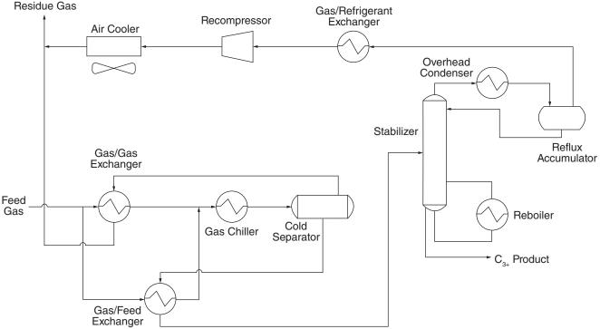
Figure C1 Example mechanical refrigeration system with stabilizer (GPSA, 2004b).
