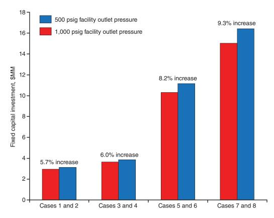
Figure 4 Effect of facility outlet pressure on the fixed capital investment. MM, million; psig, pounds per square inch gauge.
