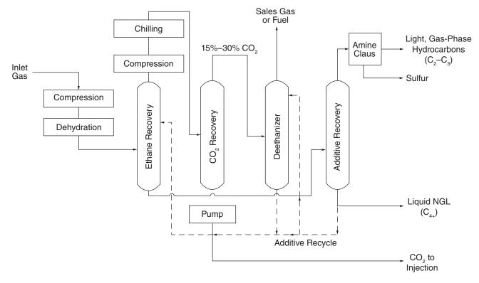
Figure C2 Typical Ryan/Holmes process flow diagram (GPSA 2004b).
