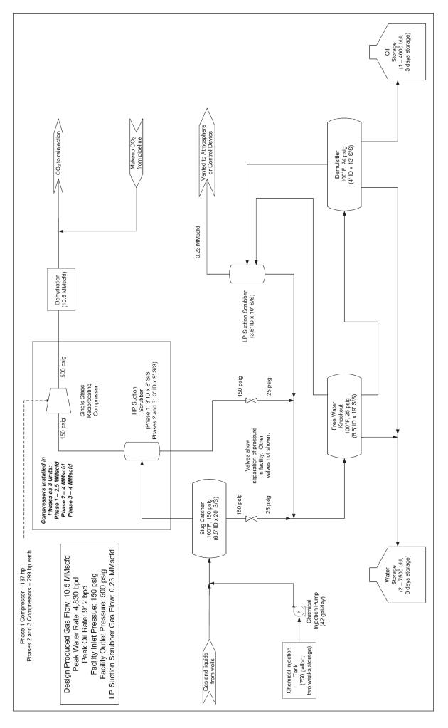
Figure A5 Process flow diagram for Case 5.
