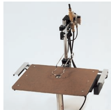
SPU7A01 Tablemount Hand Buttons Bottom Compression 1" Stroke
