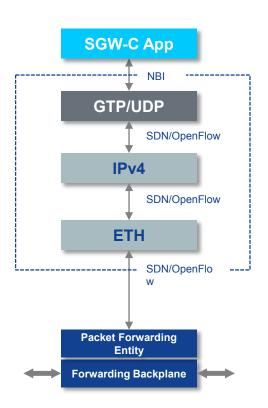
Split protocol stack along transport and adaptation/termination functions
