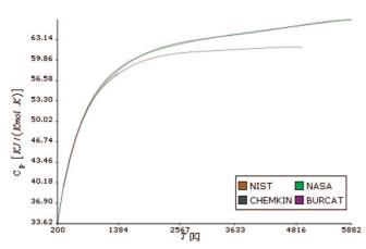
Figure 9. Plot of the standard state heat capacity of nitrogen dioxide  $(NO_2)$  showing a 5.43% difference between NASA and CHEMKIN values at 4816 K.
