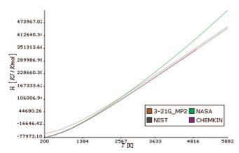
**Figure 10.** Plot of the standard state enthalpy of methane  $(CH_4)$  showing a comparison of ab initio data with that produced using the NASA nine-term and Shomate polynomials.
