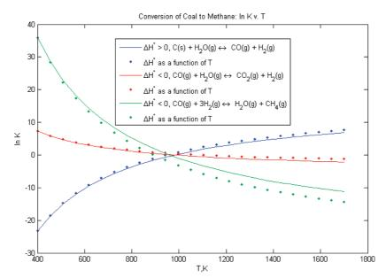
Figure 14. The MATLAB Thermochemical Data Toolbox used to plot  $\ln K$  as a function of temperature for each reaction involved in the conversion of solid coal (C(s)) to methane gas (CH<sub>4</sub>).
