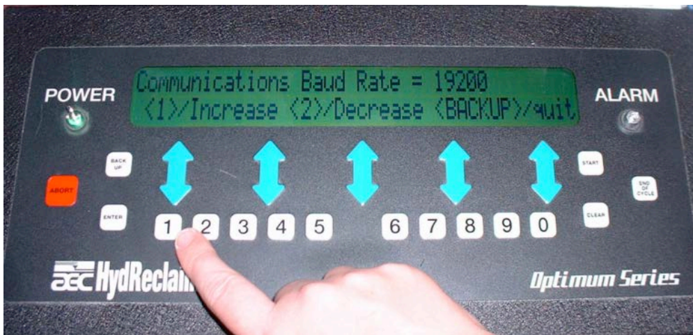
Step 5: hit "1" or "2" to change Baud Rate, then Backup
