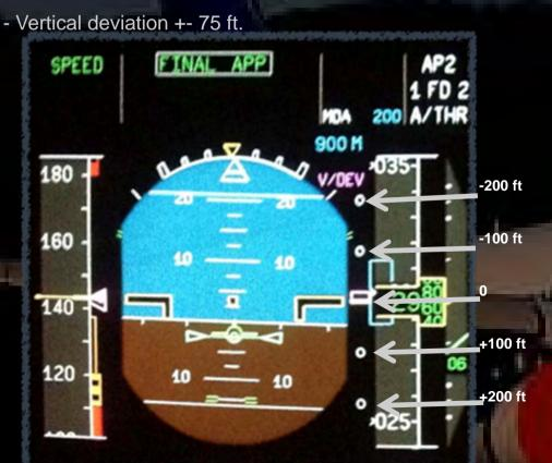
The vertical deviation scale and index appear when in approach phase and the FINAL mode is armed/engaged or a non precision approach has been entered.
