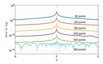
Figure 7: Error at 1000 points  $y \in [-5,5]$  in the Hilbert transform of  $u(x) = \exp(-|x|)$  computed by the global AAA-LS method from  $60, 120, \dots, 360$  exponentially spaced samples. This plot was produced in 2 secs. on a laptop.
