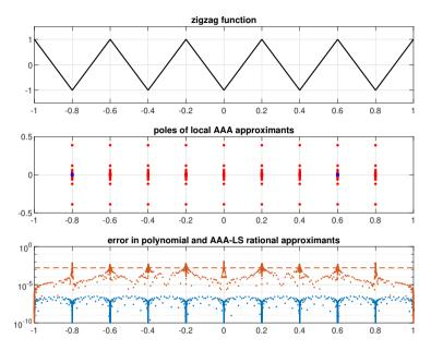
Figure 6: Top, a real zigzag function on [-1,1] to be approximated over the whole interval by a single rational function. Middle, the 466 poles determined by local AAA fits near each singularity, each of degree 51 or 52. Two poles lie in [-1,1] and are discarded (blue). Bottom, the resulting errors in the AAA-LS fit show accuracy of  $3 \times 10^{-7}$ . A polynomial with the same 962 degrees of freedom such as a Chebyshev interpolant (dots) could have accuracy at best  $10^{-3}$  (dashed line).
