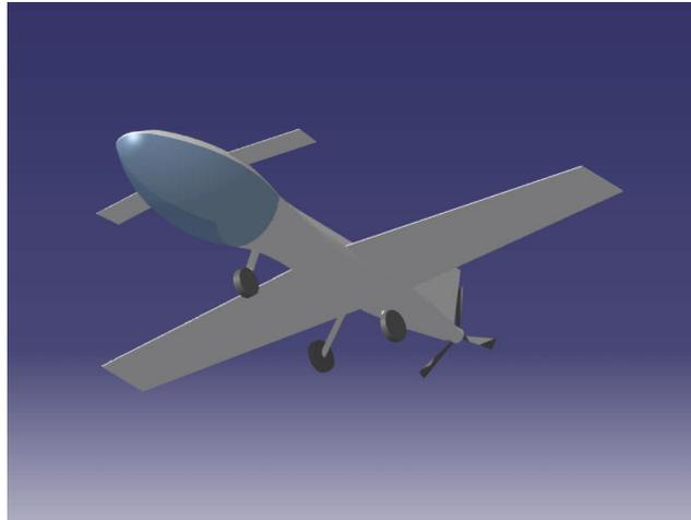
**Figure 3.7: Concept VII, Canard Pusher-prop w/ Vertical Tail**
