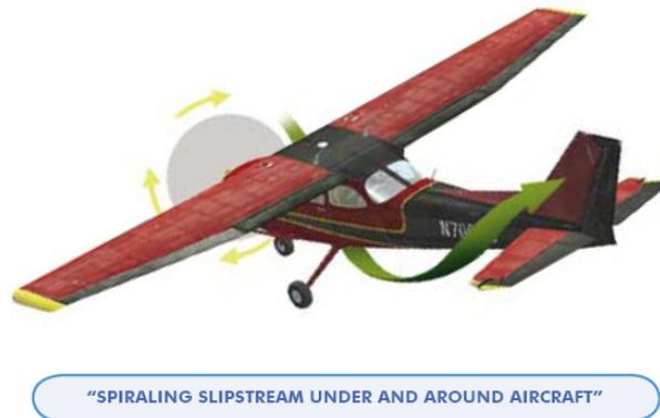
**Figure 3.1: Slipstream effect on a Cessna 172 (Image Source: <http://www.computerpilot.com/resource/files/samples/sampleArticle542.pdf>)**
