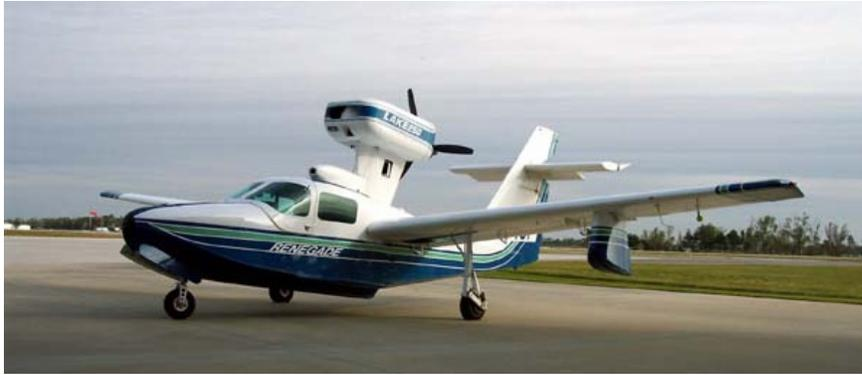
**Figure 3.2: Mid-Fuselage Mounted Engine on a Lake Renegade (Image Source: [www.teamlake.com](http://www.teamlake.com))**
