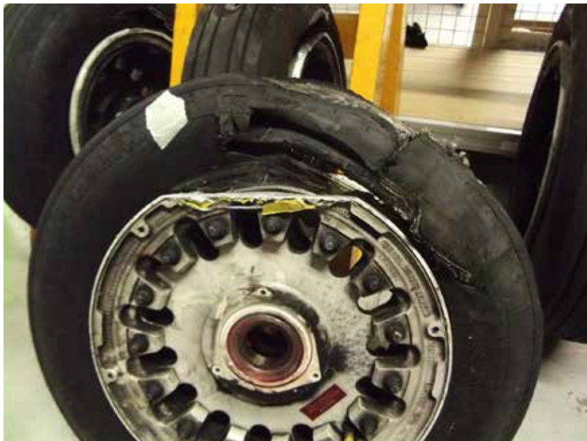
Figure 3 Right outboard wheel rim damage
