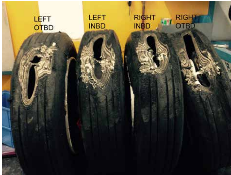
Figure 2 Damage to tyres
