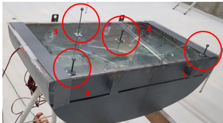
Figure 2-10: ISWEC model with Optitrack markers
