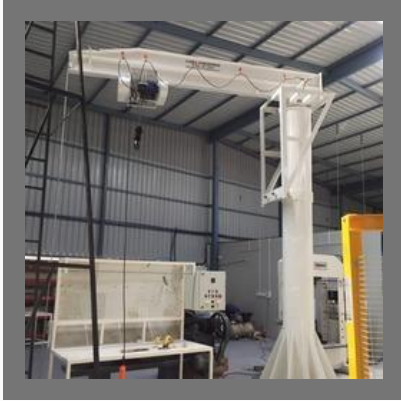
Pillar Mounted Jib Crane
