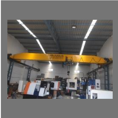
Single Beam Cranes
