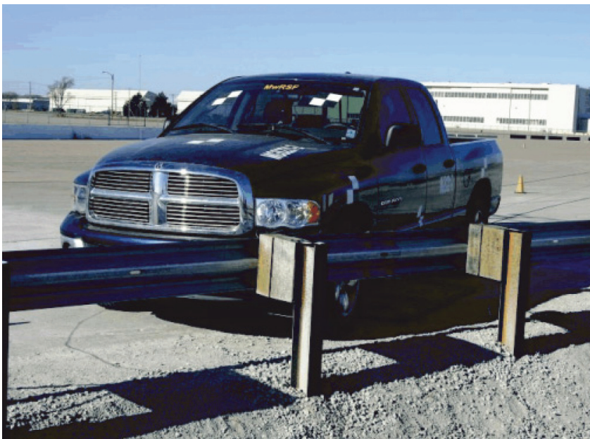
Figure 5-34. MGS Placed at 1V:2H Slope Breakpoint
