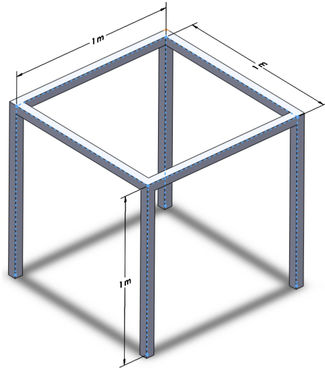
The table frame, made of steel box sections, is fixed at the end of each leg. Determine the first 10 eigenvalues and natural frequencies.
