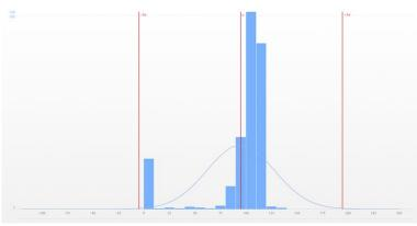
With ABB Ability<sup>TM</sup> Knowledge Manager's statistical production analysis, trend functions such as X, EWMA and CUSUM charts are selected to match specific requirements of manufacturing processes. X-Y graphs show the correlation between two variables, with compensation of time delay. Histograms allow for readable statistics of run-time quality measurements.
