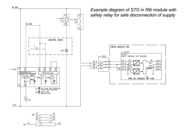
**WARNING!** The Safe torque off function does not disconnect the voltage of the main and auxiliary circuits from the drive. Therefore maintenance work on electrical parts of the drive or the motor can only be carried out after isolating the drive system from the main supply.
