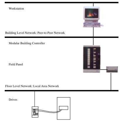
Figure:2-1 System 600 Architecture
