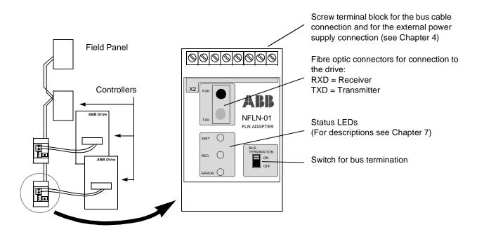
Figure 2-2 The construction of the FLN link and the NFLN-01 Adapter Module.
