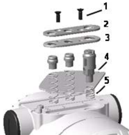
Figure 15 External push button assembly components
