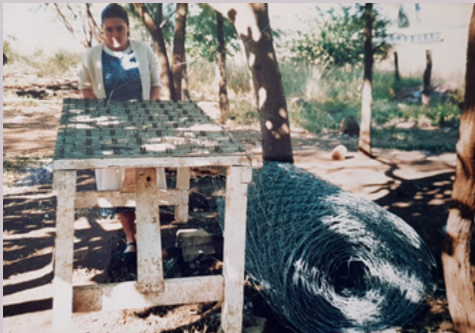
Fence-making Table. Alternative technology equipment used for an early income generating project
