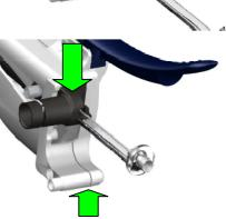
8. While pressing the two parts together, put the black inlet connector over the pin in the recess until a click is heard.
