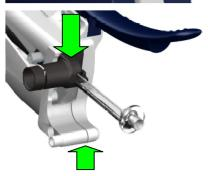
5. While pressing the two parts together, put the black inlet connector over the pin in the recess until a click is heard.
