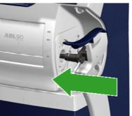
**6.** Put the inlet handle in the closed position and remount the cover.
