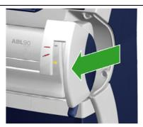
2. Lift the inlet handle to syringe position (the middle LED lights up).
