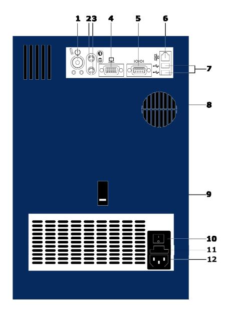
1 Standby button 2 Mouse port 3 **Keyboard port** 4 **External VGA monitor port** – for test purposes only. 5 **COM** port **Ethernet port** 6 7 **USB** ports 8 Ventilation 9 Latch for manual release of the solution pack Mains power switch – on some versions the mains power 10 switch may show "ON" and "OFF" instead of "I" and "O". 11 Fuses 12 Mains socket
