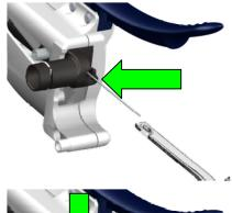
7. Place your thumb and index finger as shown and press the two parts together.
