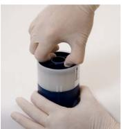
**6.** Remove the new sensor cassette by pulling it out of the sensor cassette pack with thumb and index finger.
