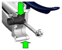
7. While pressing the two parts together, put the black inlet connector over the pin in the recess until a click is heard.
