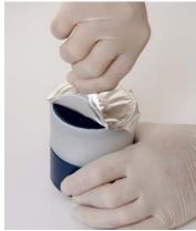
5. Screw off the revealed lid of sensor cassette pack, by screwing it off counterclockwise.
