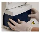
**4.** Activate the new solution pack by pulling out the safety pin.
