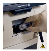
**4.** Remove the foil on top of the sensor cassette pack by pulling the foil upwards and off.
