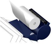
4. Make sure that some of the paper will extend out of the printer, when the cover is closed. Then close the cover by pulling the cover forwards and pressing it down until a click is heard.
