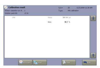
**Sens.** (cuvette factor) is a factor that expresses the ratio of the effective light path of the analyzer cuvette to that of a reference cuvette determined by Radiometer.
