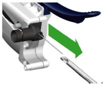
**5.** Lift the probe 90° upwards and remove it from its recess.
