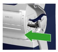
**8.** Put the inlet handle in the closed position and remount the cover.
