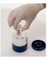
7. Holding the new sensor cassette with the thumb and index finger, press the new sensor cassette firmly into the sensor cassette seat in the sensor compartment until resistance is met.
